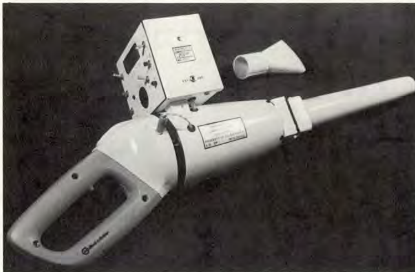
This sniffer measures airborne conductive particles as the air is drawn across an electronic grid in the flowstream. It was designed to detect carbon fibers.
